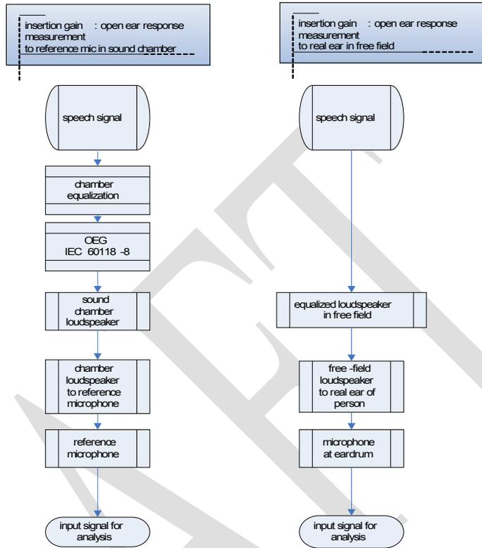
**Figure 1: Measurement set-up for open ear response for Insertion gain: Input signal. Left: proposed measurement method in sound chamber , Right: equivalent measurement method for real-ear measurement (not proposed).**
