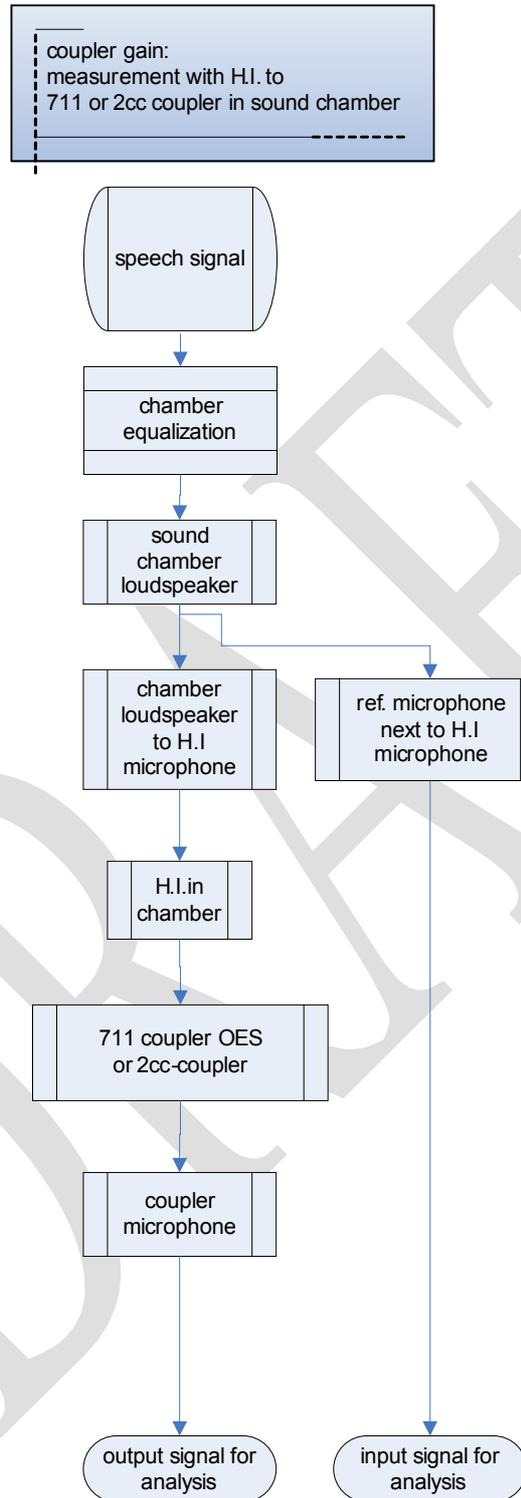
**Figure 3** Measurement set-up for Coupler gain (H.I response as well as free-field response). Proposed measurement method in sound chamber with HI to 711 coupler or 2cc coupler
