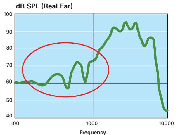
Doubling and cancelling occur at frequencies where the vent-in and amplified sounds interact at similar levels; a doubling is seen when in phase and a cancelling of sound is seen when out of phase.
