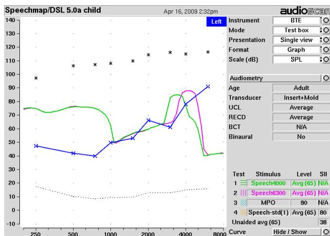
Frequency specific speech bands for 4000 Hz (green) and 6300 Hz (pink). The 6300 Hz band has been lowered to approximately 4000 Hz; 4000 Hz band has been lowered to approximately 3000 Hz. The two bands remain distinguishable from each other (with a slight amount of overlap).
