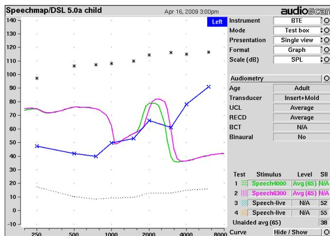
Frequency specific speech bands for 4000 Hz (green) and 6300 Hz (pink) with SoundRecover. The 6300 Hz band has been lowered to approximately 2500 Hz (similar to the /s/ sound); the 4000 Hz band has been lowered to approximately 2000 Hz. The two bands are almost entirely overlapping for this SoundRecover setting; this agrees with the live speech measurements and indicates the need for further fine-tuning of the SoundRecover setting.
