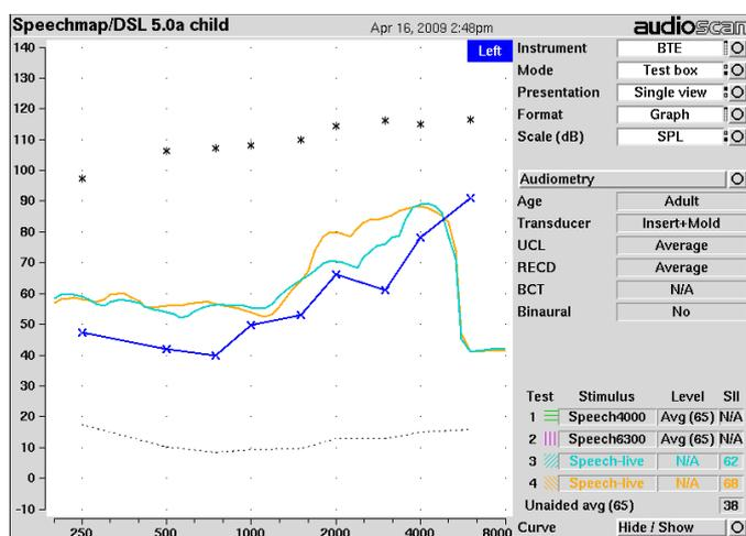
Live voice productions of /s/ (blue) and /sh/ (yellow). A distinct peak for the sound /s/ can be observed at approximately 4000 Hz. The bandwidth for the sound /sh/ is distinguishable from that of /s/ (a broader bandwidth is noted for /sh/).
