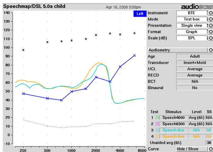
Live voice productions of /s/ (blue) and /sh/ (yellow) with SoundRecover. A distinct peak for the sound /s/ can be observed at approximately 2000 Hz. The bandwidth for the sound /sh/ is no longer entirely distinguishable from that of /s/ (the bandwidth /sh/ is much like that for /s/ for this SoundRecover setting). This indicates that the SoundRecover setting may contribute to sound confusions for this hearing loss and should be fine-tuned.
