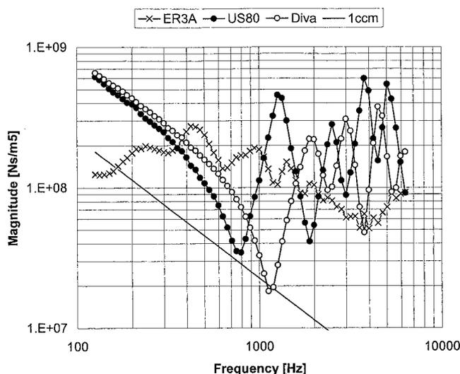
Fig. 1. Acoustic impedance of the Unitron US80, Widex Diva, and ER3 earphone compared with a 1 cc cavity.
