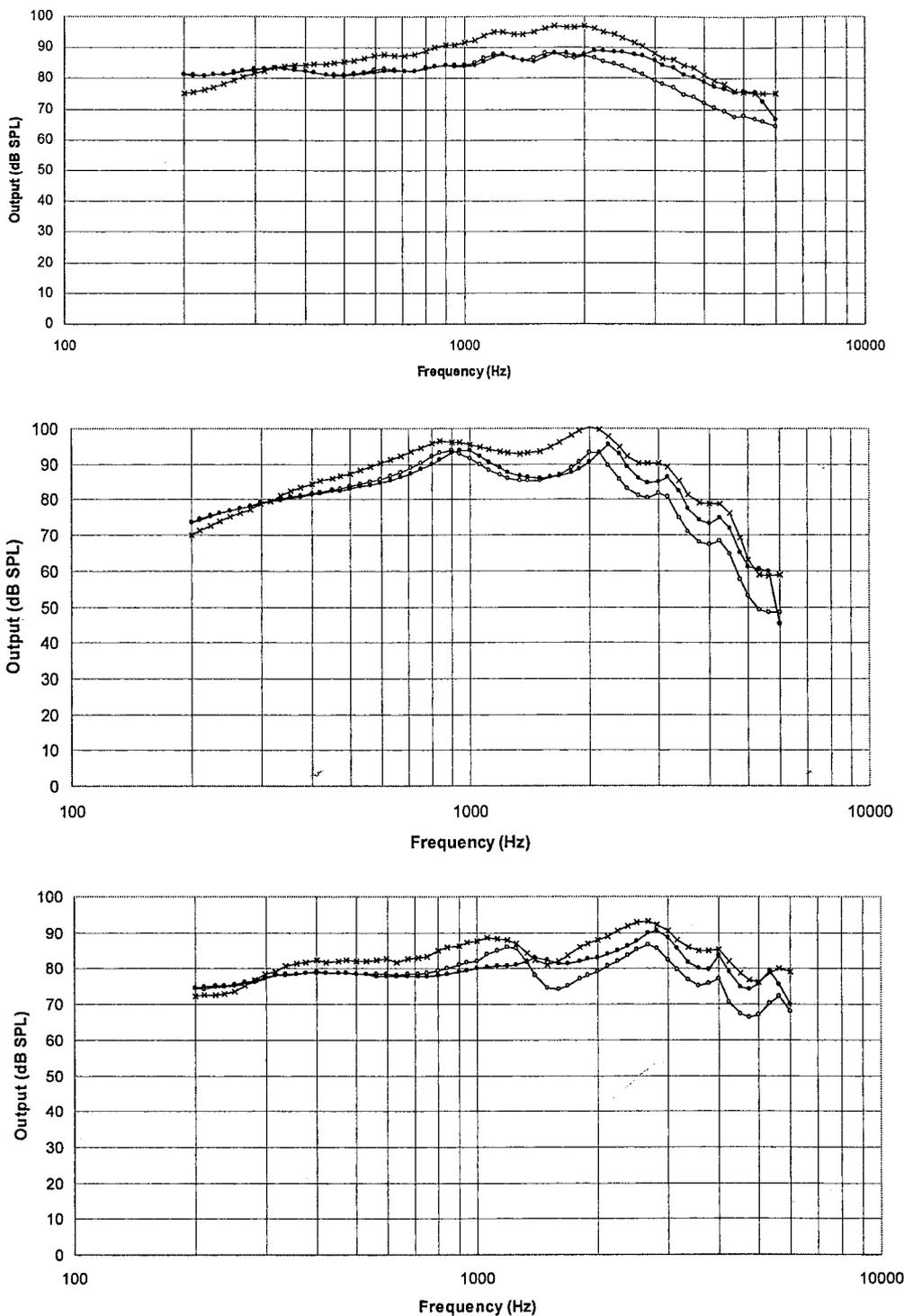
Fig. 3. Mean data measured with ER-3A (top panel), Unitron US80 (middle panel), and Widex Diva (bottom panel). Each panel shows real-ear (crosses), HA1 (open circles), and HA2 (filled) output, in SPL, as a function of frequency.
