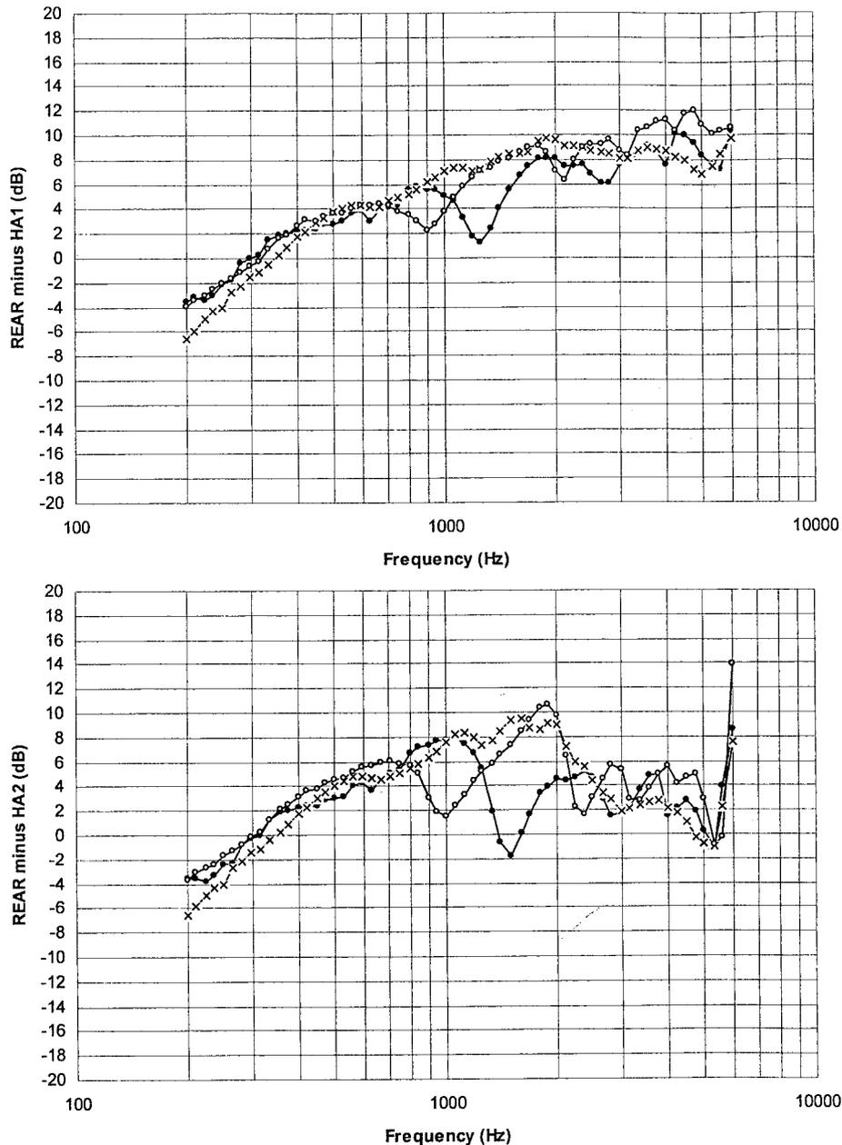
Fig. 4. Mean real-ear to coupler difference transfer function, as a function of frequency, measured with the HA1 (top panel) and HA2 (bottom panel). Each panel shows data for the ER-3A (crosses), Unitron US80 (open circles), and Widex Diva (filled circles).
