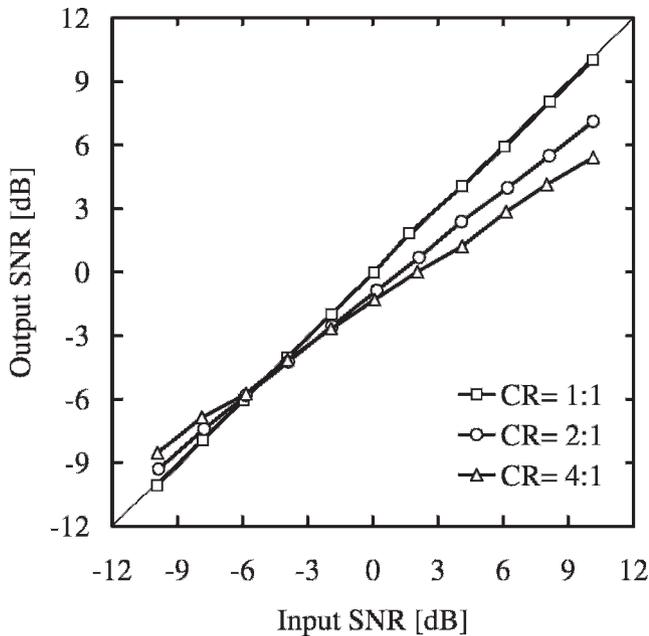
**Figure 4.** Results of measurements 4–6: signal-to-noise ratio (SNR) for single-channel fast-acting compression; compression ratios (CRs) = 1:1, 2:1, and 4:1; speech S1 in modulated noise N2.
