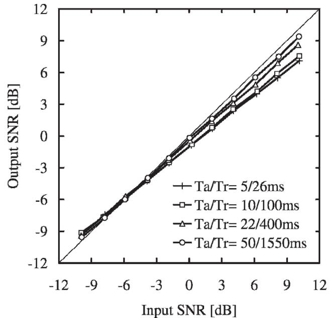
**Figure 5.** Results of measurements 7–10: signal-to-noise ratio (SNR) for single-channel compression; compression ratio 2:1; compression time constants (attack/release [Ta/Tr]) = 5/26 msec, 10/100 msec, 22/400 msec, and 50/1550 msec; speech S1 in modulated noise N2.
