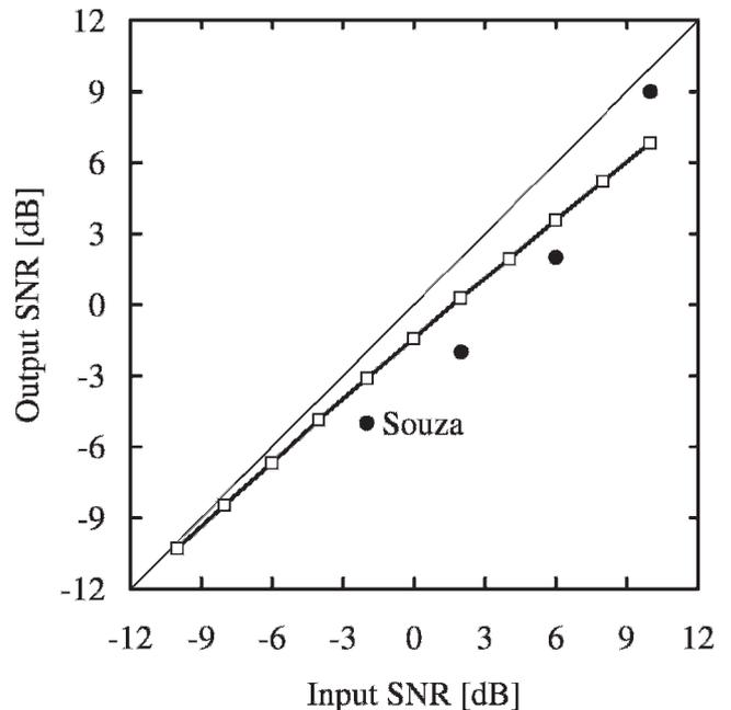
**Figure 1.** Results of measurement 1: signal-to-noise ratio (SNR) for single-channel fast-acting compression, compression ratio 2:1, speech S1 in unmodulated noise N1. Diagonal line indicates equality between Input SNR and Output SNR. Additional points (“Souza”) show data for corresponding measurement from Souza et al, 2006, Table 1.
