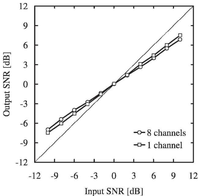
**Figure 6.** Results of measurements 11–12: signal-to-noise ratio (SNR) for single-channel and eight-channel fast-acting compression, compression ratio 2:1, speech S1 in speech N3.
