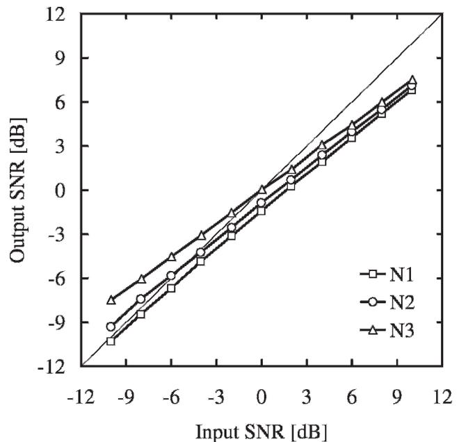
**Figure 3.** Results of measurements 1–3: signal-to-noise ratio (SNR) for single-channel fast-acting compression; compression ratio 2:1; speech S1 in unmodulated noise N1, modulated noise N2, and speech N3.
